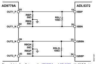
Figure 1. Interface Between the AD9779A and ADL5372 with 50  $\Omega$  Resistors to Ground to Establish the 500 mV DC Bias for the ADL5372 Baseband Inputs (Simplified Schematic)
