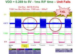
Old Part. Using Function Generator for Pulsing Unit On/OFF VDD = 0.269 to 5V - 1ms R/F time – Unit Fails
