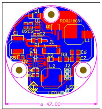
Figure 3. Revised layout of the PCB (updated from the board in Figure 2).
