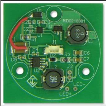
Figure 2. Photo of the PCB. The board was designed to fit directly into an MR-16 assembly.
