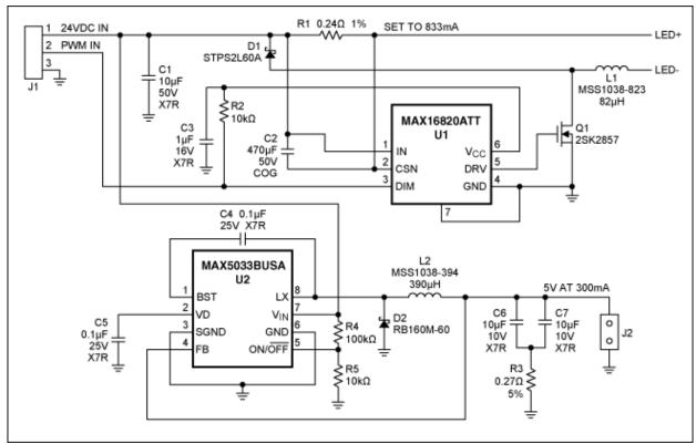
Figure 1. Schematic of the driver design.
