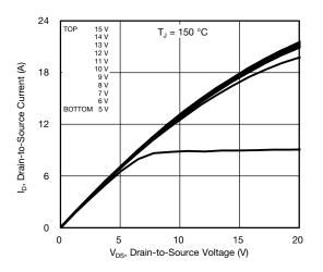
Fig. 2 - Typical Output Characteristics
