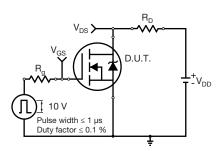
Fig. 13 - Switching Time Test Circuit
