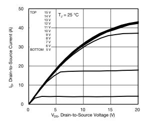
Fig. 1 - Typical Output Characteristics
