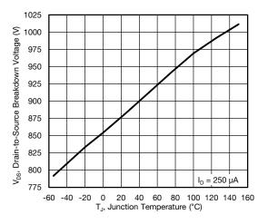
Fig. 11 - Temperature vs. Drain-to-Source Voltage
