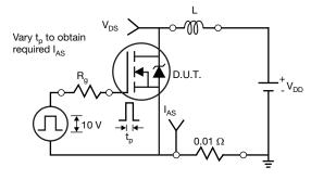
Fig. 15 - Unclamped Inductive Test Circuit
