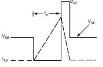
Fig. 16 - Unclamped Inductive Waveforms
