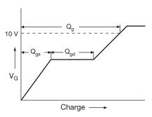
Fig. 17 - Basic Gate Charge Waveform
