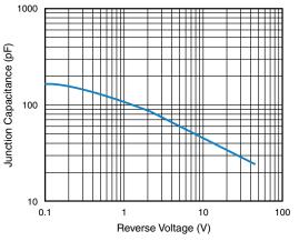
Fig. 5 - Typical Junction Capacitance
