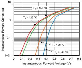
Fig. 3 - Typical Instantaneous Forward Characteristics
