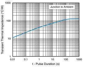
Fig. 6 - Typical Transient Thermal Impedance
