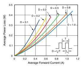
Fig. 2 - Forward Power Loss Characteristics
