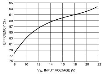
Figure 24. Efficiency vs. Input Voltage for the Boost Demo Board at  $I_{OUT}$  = 350 mA,  $V_{OUT}$  = 22 V (6xLED with V<sub>F</sub> = 3.6 V), T<sub>A</sub> = 25°C
