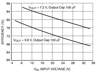
Figure 21. Efficiency vs. Input Voltage for the 1.5 A Buck Demo Board at  $I_{out}$  = 700 mA,  $T_A$  = 25°C, with 100  $\mu$ F Output Capacitor
