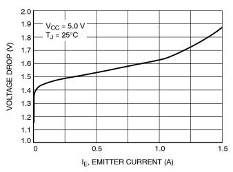
Figure 9. Emitter Follower Configuration Output Darlington Switch Voltage Drop vs. Emitter Current
