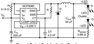
Figure 1. Typical Buck Application Circuit
