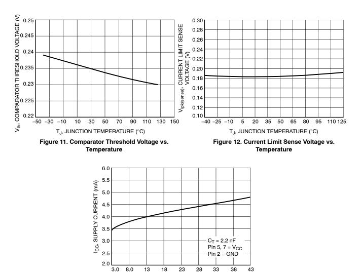
V<sub>CC</sub>, SUPPLY VOLTAGE (V) Figure 13. Standby Supply Current vs. Supply Voltage
