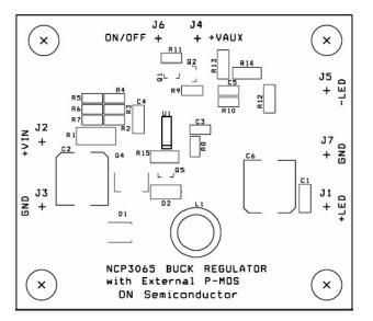
Figure 18. 1.5 A Buck Demoboard Layout
