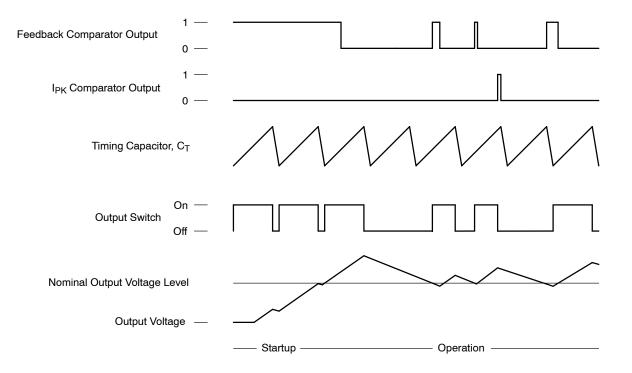
Figure 14. Typical Operating Waveforms
