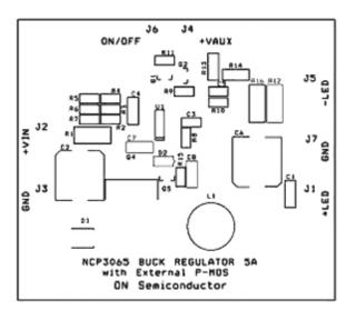
Figure 26. 3 A Buck Demoboard Layout
