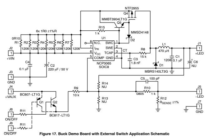
This design illustrates the NCP3065 being used as a PFET controller, the design has been optimized for continuous current operation with low ripple which allows the output filter capacitor to be eliminated. Figure 20 illustrates the
