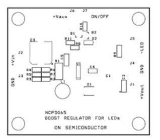
Figure 23. Boost Demoboard Layout
