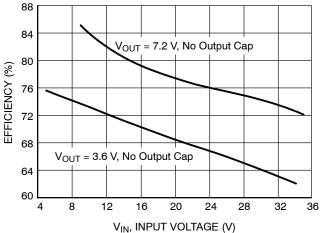
Figure 19. Efficiency vs. Input Voltage for the 1.5 A Buck Demo Board at  $I_{out}$  = 700 mA,  $T_A$  = 25°C, Without Output Capacitor
