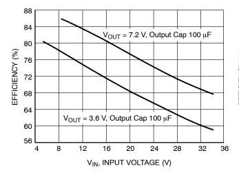
Figure 20. Efficiency vs. Input Voltage for the 1.5 A Buck Demo Board at I<sub>out</sub> = 350 mA, T<sub>A</sub> = 25°C, with 100  $\mu$ F Output Capacitor
