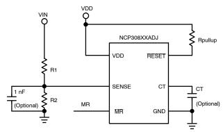
Figure 12. Using NCP308XXADJ to Monitor a User-Defined Threshold Voltage
