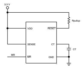
Figure 16. Delay Time Set by Capacitor
