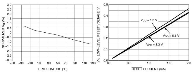
Figure 10. Normalized Sense Threshold Voltage (V<sub>IT</sub>) vs. Temperature
