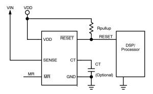
Figure 2. Typical Application Circuit for Fixed Versions
