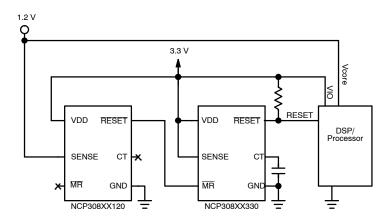
Figure 13. Using MR to Monitor Multiple System Voltages
