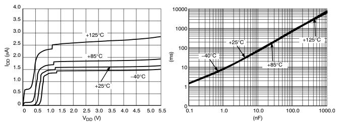
Figure 6. Supply Current vs. Input Voltage
