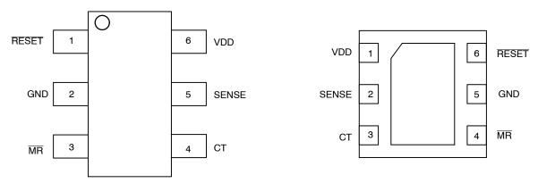
Figure 4. Pin Connections Diagram (Top View)
