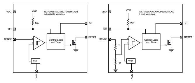
Figure 3. Functional Block Diagrams of Adjustable and Fixed Versions
