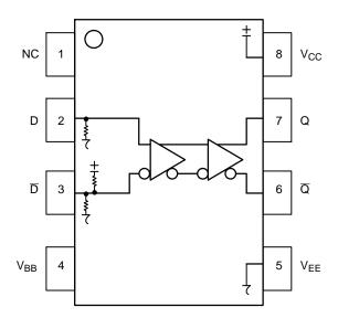
Figure 1. Logic Diagram and Pinout Assignment
