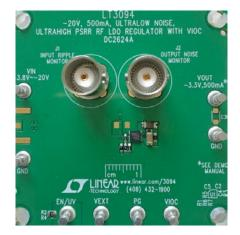
Figure 2. Demo circuit shows a tiny -3.3 V solution.
