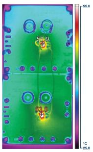
Figure 4. Thermal image of two paralleled LT3094s.
