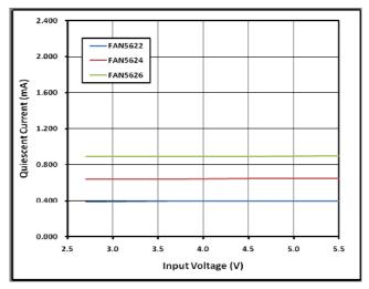
Figure 12. Shutdown Current vs. Input Voltage
