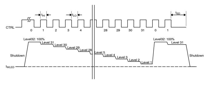
Figure 17. Digital Pulse Dimming Control Diagram
