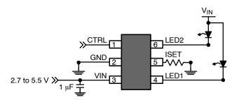
Figure 1. Typical Application of FAN5622
