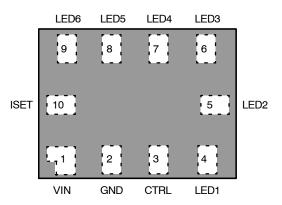
Figure 7. FAN5626: 10-Lead MicroPak MLP, Top View
