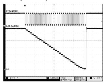
Figure 16. Dimming Operation
