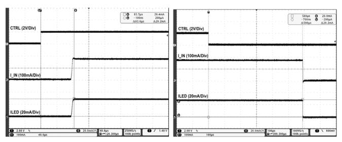
Figure 14. Startup Waveform for FAN5626
