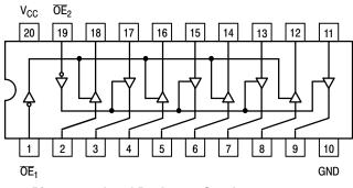
Pinout: 20-Lead Packages Conductors (Top View)
