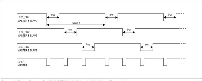
Figure 23. Timing Diagram for GPIO CTRL[3:0] 0110 and 1000 Without External Mux
