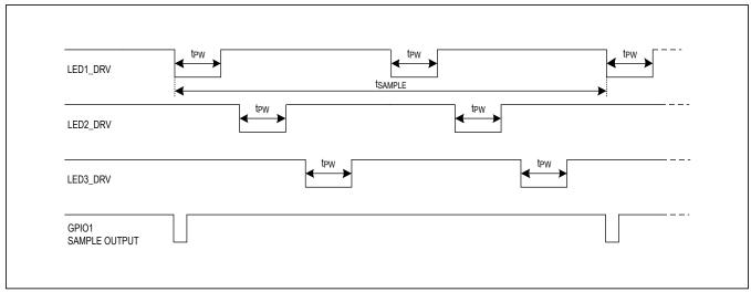
Figure 19. Timing Diagram for GPIO CTRL[3:0] 0101
