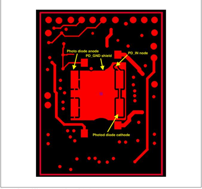
Figure 32. Example PCB Layout, Layer 6 (Bottom, Optical Layer)
