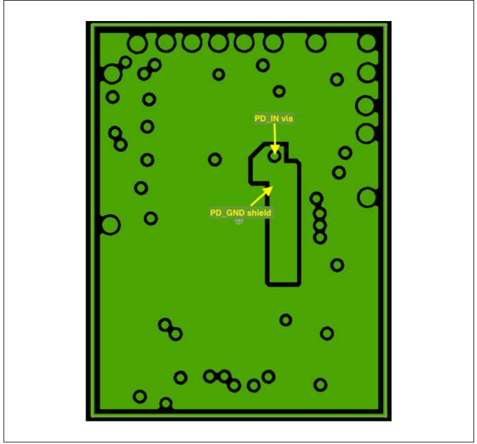
Figure 33. Example PCB Layout, Layer5 (Ground Layer)
