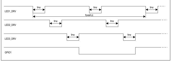
Figure 9. Timing Diagram for GPIO CTRL[3:0] 0000 and 0001 with External Mux
