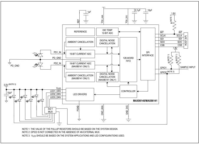
Figure 25. Block Diagram for GPIO CTRL[3:0] 1010
