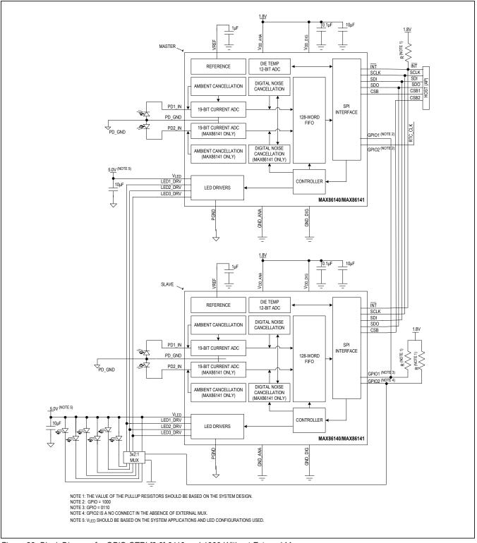
Figure 22. Block Diagram for GPIO CTRL[3:0] 0110 and 1000 Without External Mux
