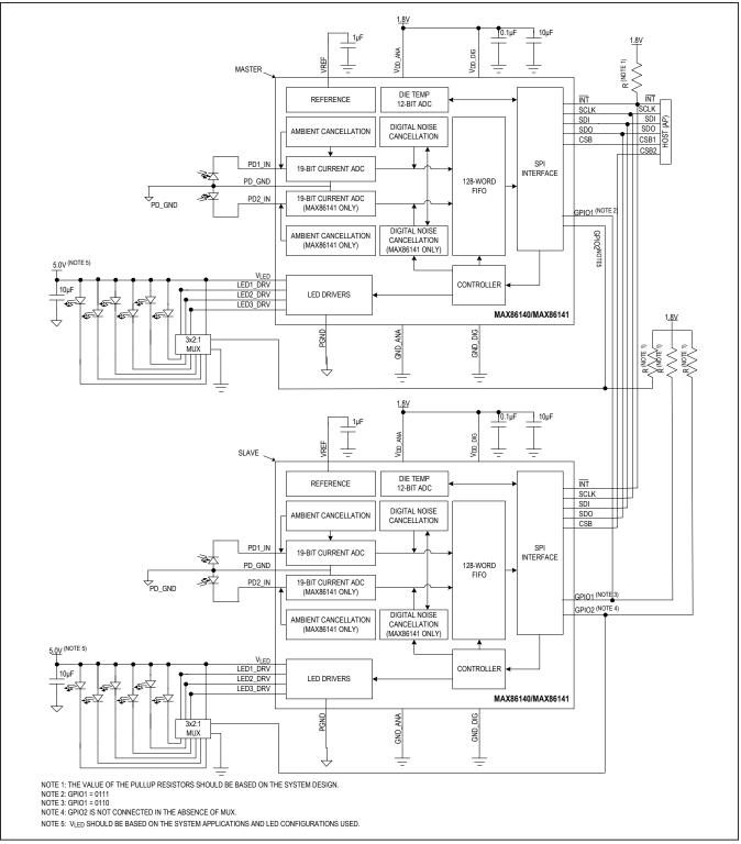
Figure 20. Block Diagram for GPIO CTRL[3:0] 0110 and 0111 With Two External Muxes
