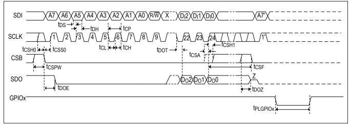
Figure 34. Detailed SPI Timing Diagram
