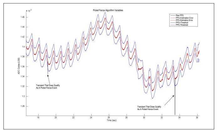
Figure 30. Picket Fence Variables In A PPG Waveform
