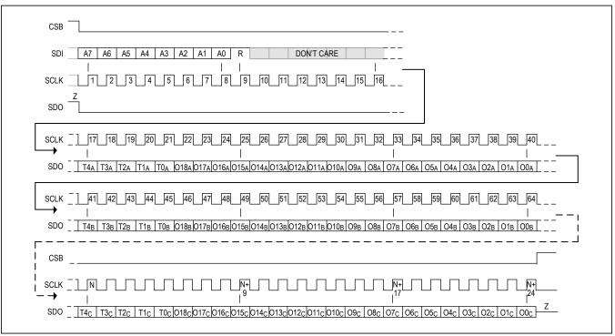
Figure 37. SPI FIFO Burst Mode Read Transaction
