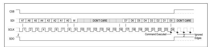
Figure 35. SPI Write Transaction
