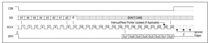
Figure 36. SPI Read Transaction
