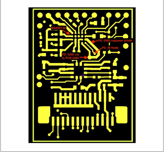
Figure 31. Example PCB Layout, Layer 1 (Top, MAX86140)
