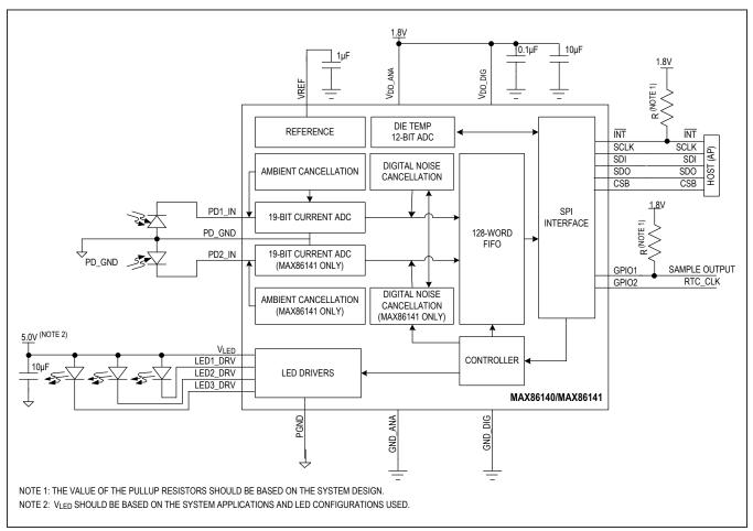
Figure 18. Block Diagram for GPIO CTRL[3:0] 0101
