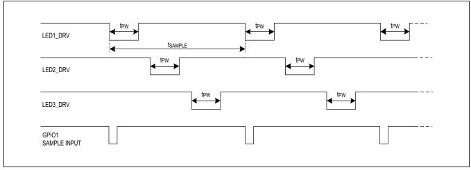
Figure 14. Timing Diagram for GPIO CTRL[3:0] 0011
