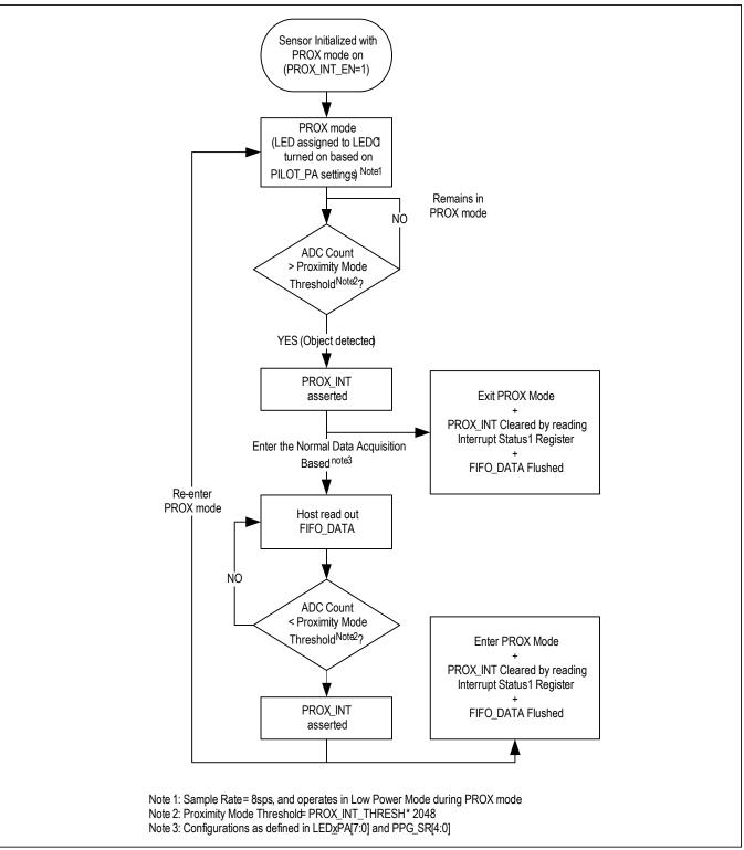
Figure 28. Proximity Function Flow Diagram
