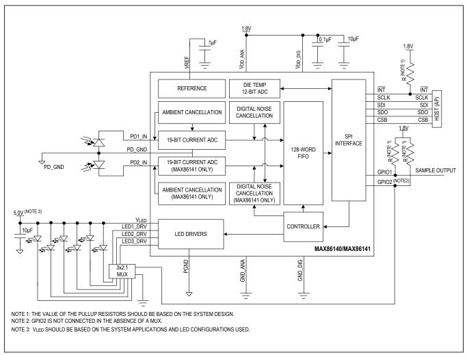
Figure 15. Block Diagram for GPIO CTRL[3:0] 0100 Without External Mux
