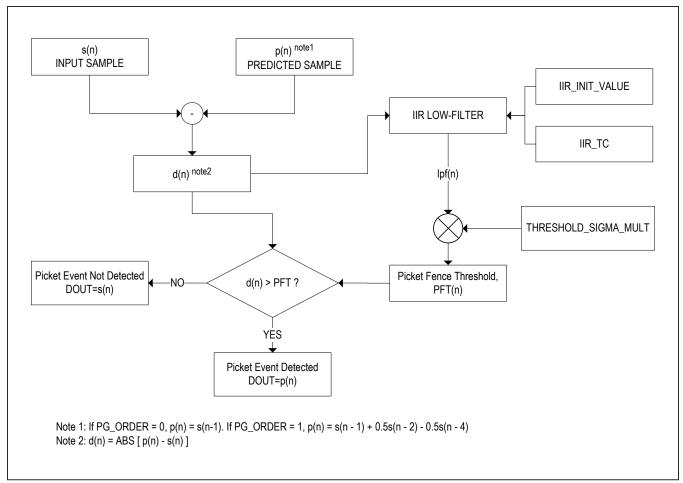
Figure 29. Picket Fence Detect-and-Replace Function Flow
