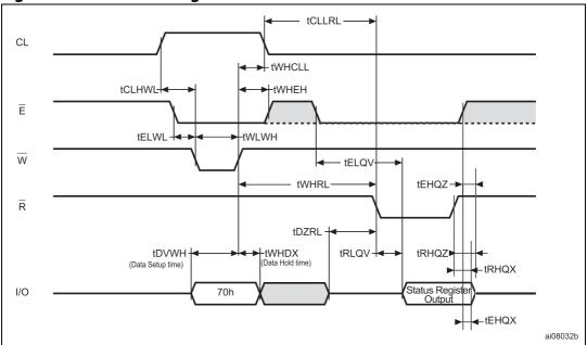
Figure 25. Read status register AC waveform
