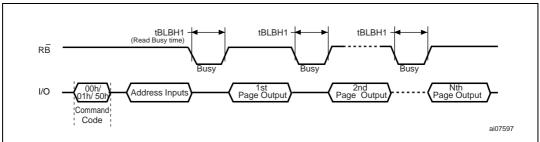
Figure 13. Sequential row read block diagrams
