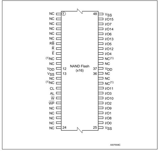
Figure 4. TSOP48 connections, x16 devices
