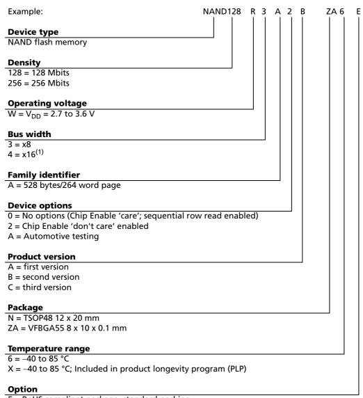
E = RoHS compliant package, standard packing F = RoHS compliant package, tape and reel packing
