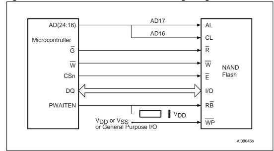
Figure 38. Connection to microcontroller, without glue logic
