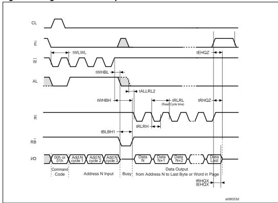
Figure 27. Page read A/read B operation AC waveform
