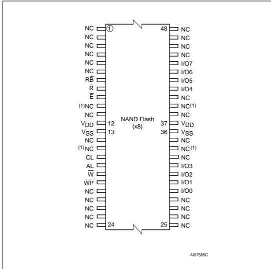
Figure 3. TSOP48 connections, x8 devices
