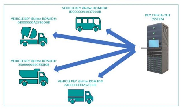
Figure 3. iButton device usage in asset tracking.
