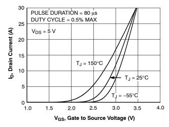
Figure 5. Transfer Characteristics
