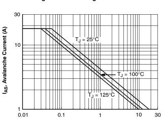
Figure 9. Unclamped Inductive Switching Capability
