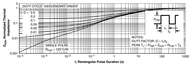
Figure 13. Junction-to-Ambient Transient Thermal Response Curve
