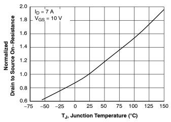
Figure 3. Normalized On–Resistance vs. Junction Temperature
