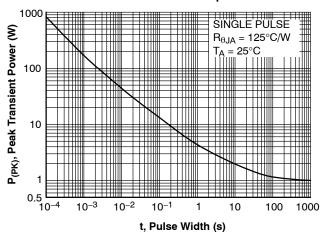
Figure 12. Single Pulse Maximum Power Dissipation
