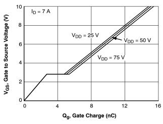
Figure 7. Gate Charge Characteristics
