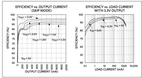
Figure 1. Efficiency for the MAX15053 switching regulator (left) versus the MAX1556 step-down regulator (right). Data shows that the MAX1556 would be a better choice for always-on power in standby mode.
