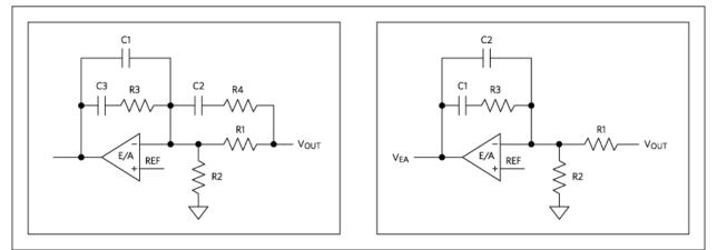
Figure 5. Schematics showing VM compensation (left) versus CM compensation (right). With CM compensation, C2 may not be needed.
