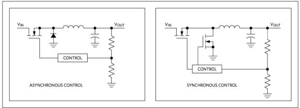
Figure 6. Asynchronous versus synchronous control.
