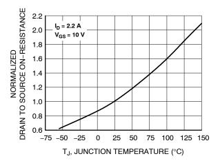
Figure 3. Normalized On-Resistance vs Junction Temperature
