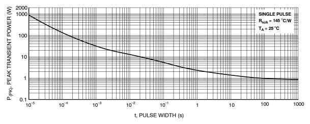
Figure 11. Single Pulse Maximum Power Dissipation
