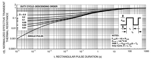
Figure 12. Junction to Ambient Transient Thermal Response Curve
