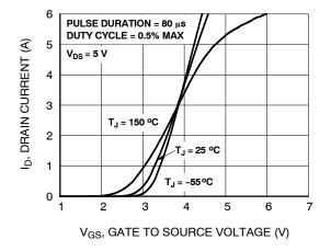
Figure 5. Transfer Characteristics
