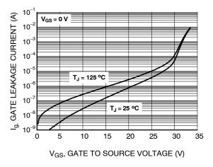
Figure 9. Gate Leakage Current vs.
