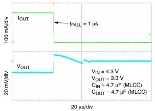
Figure 31. Load Transient Response – Falling Edge, V<sub>OUT</sub> = 3.3 V, I<sub>OUT</sub> = 1 mA to 300 mA
