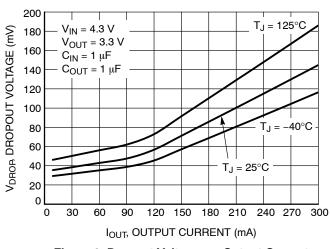
Figure 9. Dropout Voltage vs. Output Current
