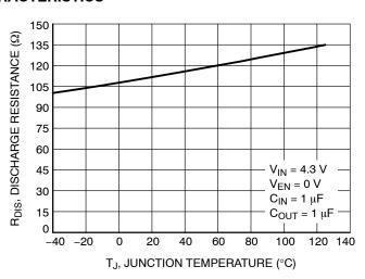
Figure 16. Discharge Resistance vs. **Temperature**
