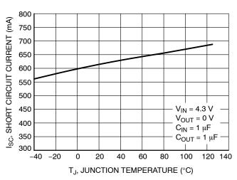
Figure 12. Short Circuit Current vs. Temperature
