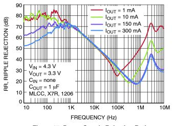
Figure 17. Power Supply Rejection Ratio - $C_{OUT} = 1 \mu F$
