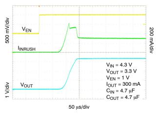
Figure 23. Enable Turn-on Response –  $C_{OUT}$  = 4.7  $\mu$ F,  $I_{OUT}$  = 300 mA
