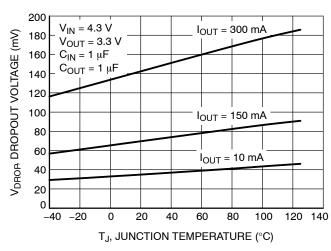
Figure 10. Dropout Voltage vs. Temperature
