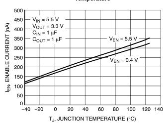
Figure 14. Current to Enable Pin vs. Temperature
