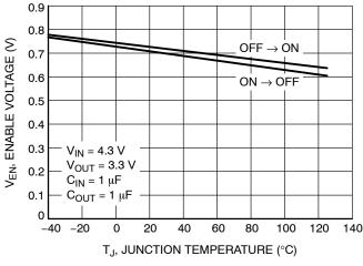
Figure 13. Enable Voltage Threshold vs.
