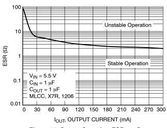
Figure 18. Output Capacitor ESR vs. Output Current
