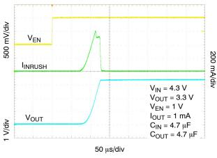
Figure 22. Enable Turn-on Response –  $C_{OUT} = 4.7 \mu F$ ,  $I_{OUT} = 1 mA$
