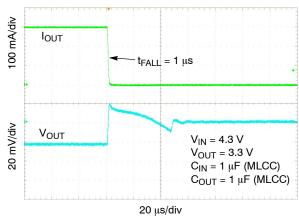
Figure 29. Load Transient Response – Falling Edge, V<sub>OUT</sub> = 3.3 V, I<sub>OUT</sub> = 1 mA to 300 mA
