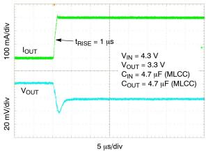
Figure 30. Load Transient Response – Rising Edge, V<sub>OUT</sub> = 3.3 V, I<sub>OUT</sub> = 1 mA to 300 mA
