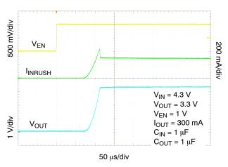
Figure 21. Enable Turn-on Response –  $C_{OUT}$  = 1  $\mu$ F,  $I_{OUT}$  = 300 mA
