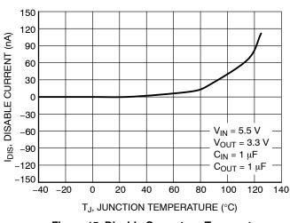
Figure 15. Disable Current vs. Temperature
