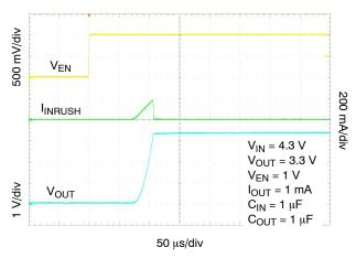
Figure 20. Enable Turn-on Response –  $C_{OUT}$  = 1  $\mu$ F,  $I_{OUT}$  = 1 mA
