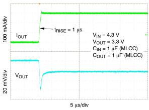
Figure 28. Load Transient Response – Rising Edge, V<sub>OUT</sub> = 3.3 V, I<sub>OUT</sub> = 1 mA to 300 mA
