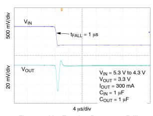
Figure 27. Line Transient Response – Falling Edge, I<sub>OUT</sub> = 300 mA
