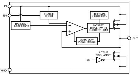
\*Active output discharge function is present only in NCV8114ASNyyyTCG devices. yyy denotes the particular  $V_{OUT}$  option.
