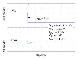
Figure 25. Line Transient Response – Falling Edge, I<sub>OUT</sub> = 1 mA
