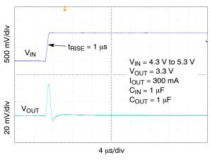
Figure 26. Line Transient Response – Rising Edge, I<sub>OUT</sub> = 300 mA
