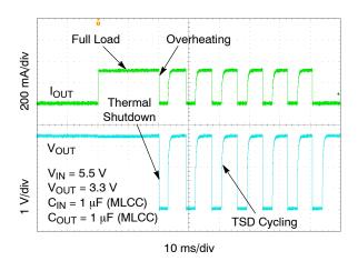
Figure 33. Short Circuit and Thermal Shutdown
