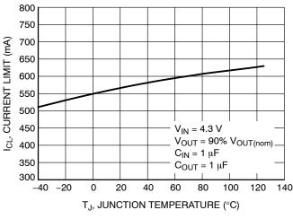
Figure 11. Current Limit vs. Temperature
