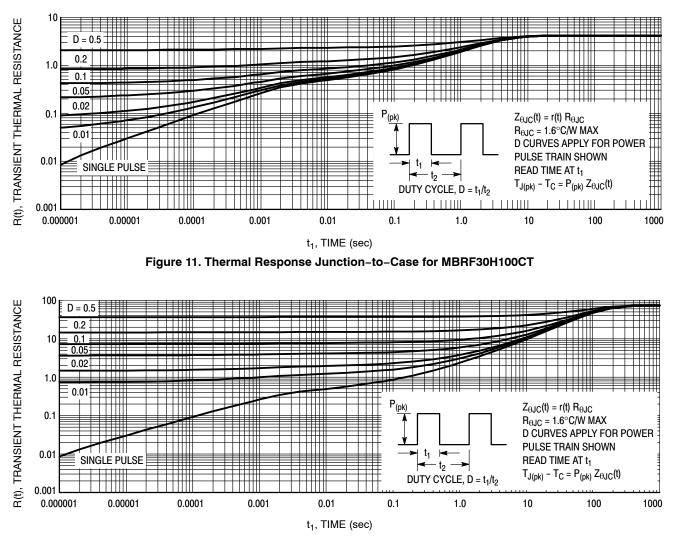
Figure 12. Thermal Response Junction-to-Ambient for MBRF30H100CT
