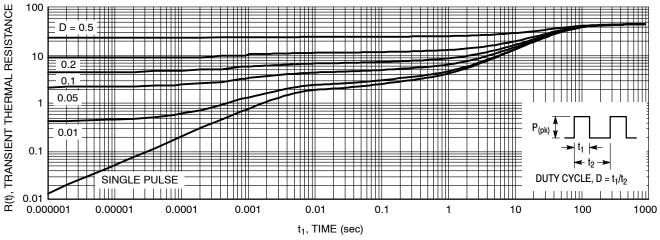
Figure 9. Thermal Response Junction-to-Ambient for MBR30H100CT
