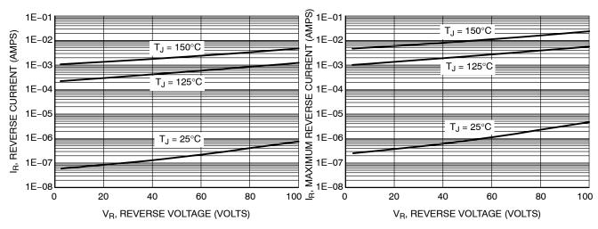
Figure 3. Typical Reverse Current
