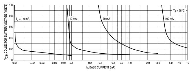
Figure 15. Collector Saturation Region
