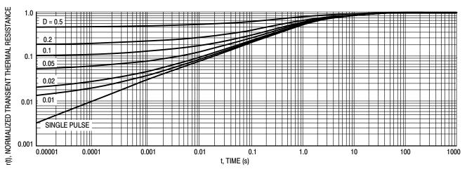
**Figure 1. Normalized Thermal Response**
