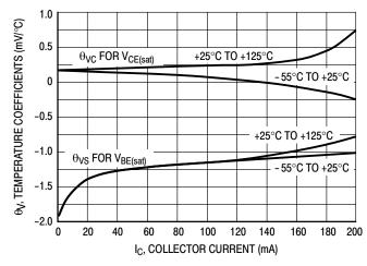
Figure 17. Temperature Coefficients
