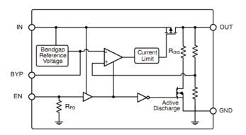
Figure 2. Simplified Block Diagram
