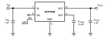
Figure 1. NCP700B Typical Application (WDFN6)
