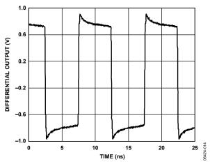
Figure 19. LVPECL Output (Differential) at 100 MHz
