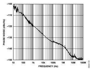
Figure 35. Phase Noise (Additive) LVDS at 800 MHz, Divide-by-2
