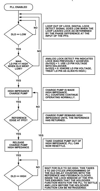
Figure 53. Flowchart of Automatic/Internal Holdover Mode
