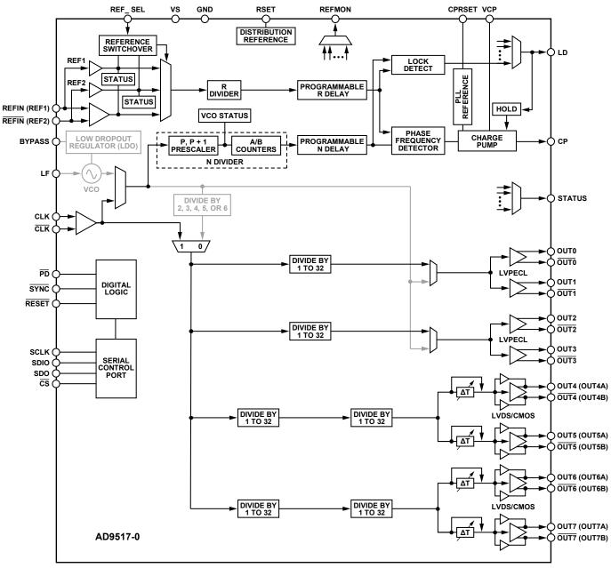
Figure 45. Clock Distribution or External VCO < 1600 MHz
