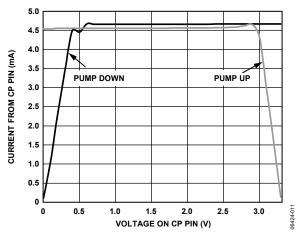
Figure 11. Charge Pump Characteristics at  $V_{CP} = 3.3 \text{ V}$
