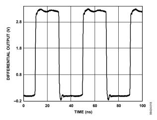
Figure 23. CMOS Output at 25 MHz
