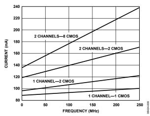
Figure 9. Current vs. Frequency—CMOS Outputs
