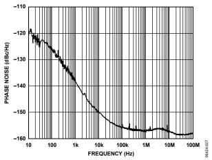
Figure 32. Phase Noise (Additive) LVPECL at 200 MHz, Divide-by-5
