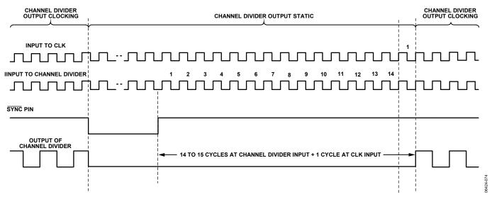
Figure 58. SYNC Timing When VCO Divider Is Not Used—CLK Input Only
