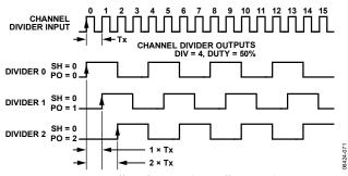
Figure 55. Effect of Coarse Phase Offset (or Delay)
