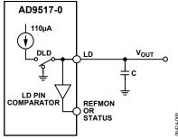
Figure 51. Current Source Lock Detect
