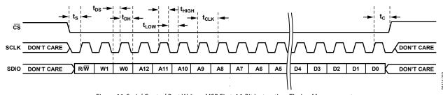
$\textit{Figure 66. Serial Control Port Write} \\ -- \textit{MSB First, 16-Bit Instruction, Timing Measurements} \\$
