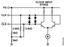
Figure 52. CLK Equivalent Input Circuit
