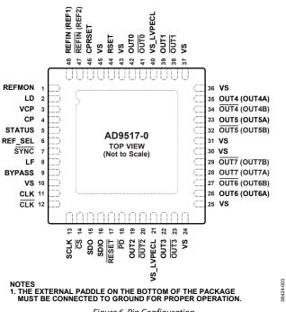
Figure 6. Pin Configuration
