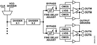
Figure 56. Fine Delay (OUT4 to OUT7)
