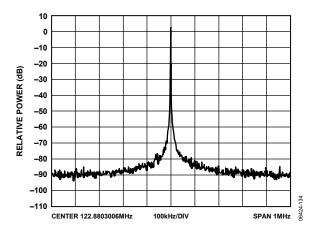
Figure 18. Output Spectrum, LVDS; 122.88 MHz; PFD = 15.36 MHz; LBW = 190 kHz;  $I_{CP}$  = 4.2 mA;  $I_{VCO}$  = 2.7 GHz
