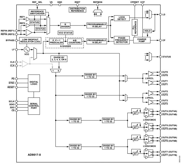
Figure 44. Internal VCO and Clock Distribution
