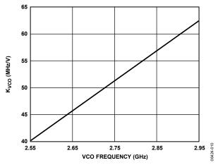
Figure 10. VCO K<sub>VCO</sub> vs. Frequency
