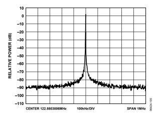
Figure 17. Output Spectrum, LVPECL; 122.88 MHz; PFD = 15.36 MHz; LBW = 190 kHz;  $I_{CP}$  = 4.2 mA;  $I_{VCO}$  = 2.7 GHz
