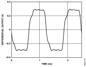
Figure 22. LVDS Output (Differential) at 800 MHz
