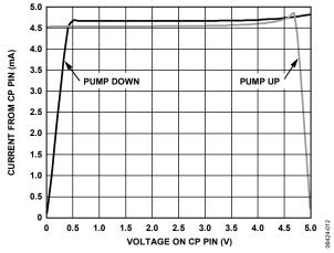
Figure 12. Charge Pump Characteristics at  $V_{CP} = 5.0 \text{ V}$
