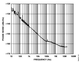
Figure 36. Phase Noise (Additive) CMOS at 50 MHz, Divide-by-20
