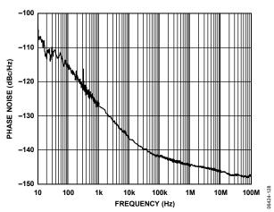
Figure 33. Phase Noise (Additive) LVPECL at 1600 MHz, Divide-by-1
