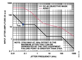
Figure 41. GR-253 Jitter Tolerance Plot
