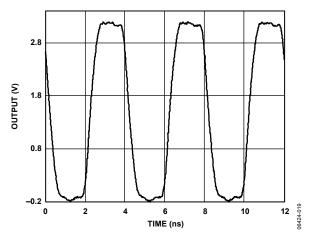
Figure 24. CMOS Output at 250 MHz
