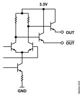
Figure 59. LVPECL Output Simplified Equivalent Circuit
