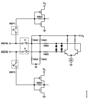
Figure 49. REFIN Equivalent Circuit
