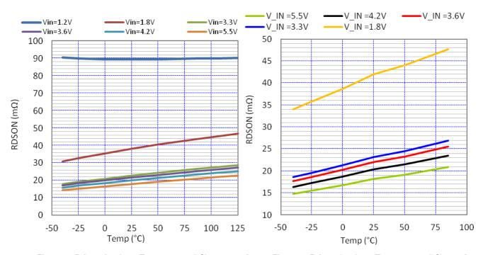
Figure 6. Rdson (m $\Omega$ ) vs. Temperature (°C) at 100 mA
