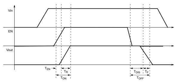
Figure 3. Enable, Rise and Fall Time
