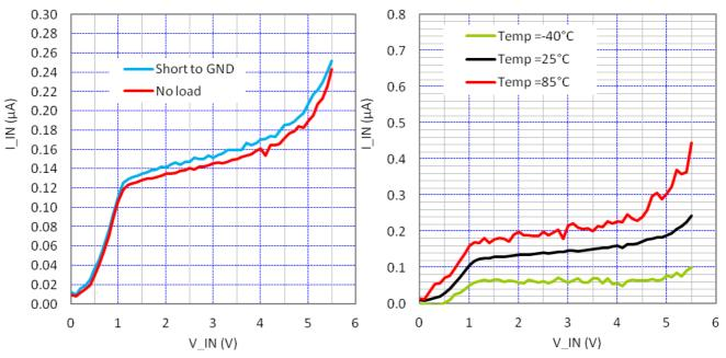
Figure 8. Standby ( $\mu A$ ) and Leakage Current ( $\mu A$ ) vs. Vin (V)
