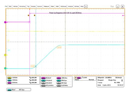
Figure 12. Enable Time and Rise Time
