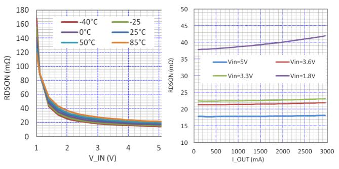
Figure 4. Rdson (m $\Omega$ ) vs. Vin (V)
