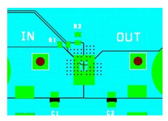
Figure 14. Routing Example: 2 oz, 4 layers with vias across 2 internal inners.
