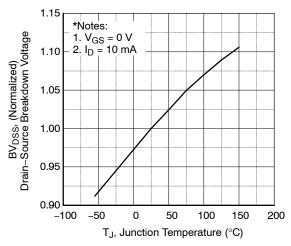
Figure 7. Breakdown Voltage Variation vs. Temperature
