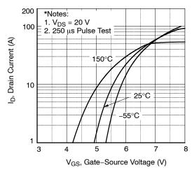
Figure 2. Transfer Characteristics
