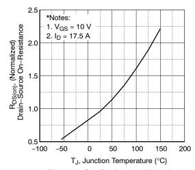
Figure 8. On–Resistance Variation vs. Temperature
