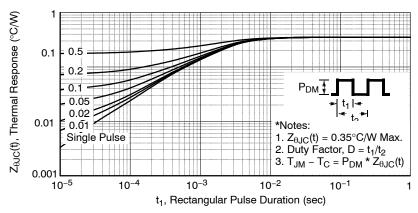
Figure 12. Transient Thermal Response Curve
