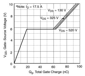
Figure 6. Gate Charge Characteristics
