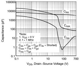
Figure 5. Capacitance Characteristics
