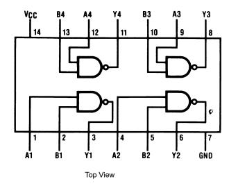
Figure 1. Pin Assignments for TSSOP
