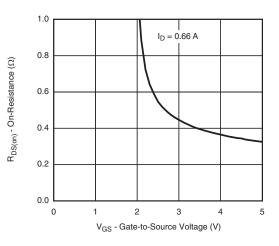
On-Resistance vs. Gate-to-Source Voltage
