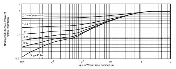
Normalized Thermal Transient Impedance, Junction-to-Foot
