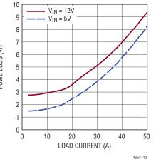
Figure 12. 1.5V Output Power Loss
