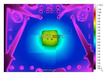
Figure 10. Thermal Image 12V to 1V, 50A with No Airflow and No Heat Sink (Based on 4-Layer 101mm × 114mm PCB Board Containing 2oz Copper on the Top, Bottom and All Internal Layers)
