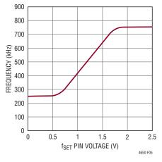
Figure 5. Operating Frequency vs  $f_{\text{SET}}$  Pin Voltage
