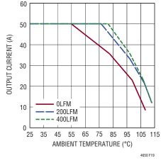
Figure 19. 5V to 1.5V Derating Curve, BGA Heat Sink
