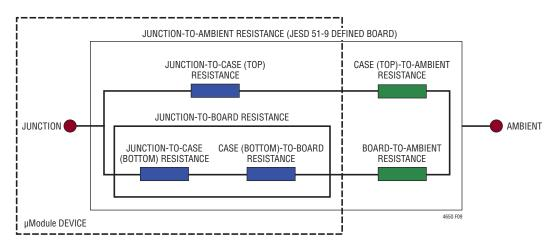
Figure 9. Graphical Representation of JESD51-12 Thermal Coefficients
