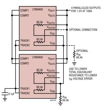
Figure 2. 4-Phase Parallel Configurations
