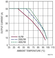
Figure 18. 12V to 1.5V Derating Curve, No Heat Sink
