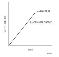
Figure 7. Output Coincident Tracking Waveform
