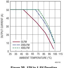
Figure 20. 12V to 1.5V Derating Curve, BGA Heat Sink
