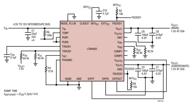
Figure 6. Example of Output Tracking Application Circuit
