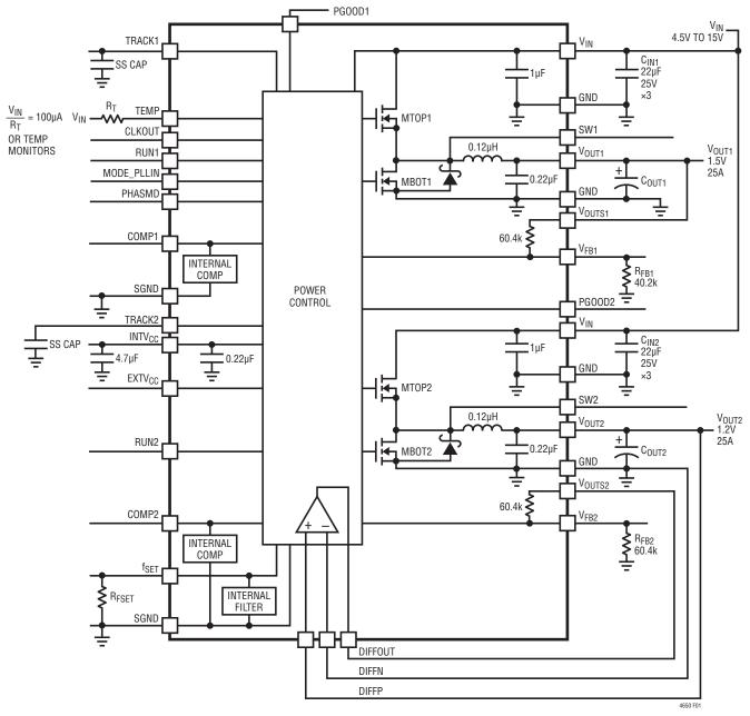
Figure 1. Simplified LTM4650 Block Diagram
