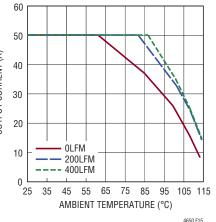
Figure 15. 5V to 0.9V Derating Curve, BGA Heat Sink
