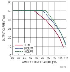
Figure 13. 5V to 0.9V Derating Curve, No Heat Sink
