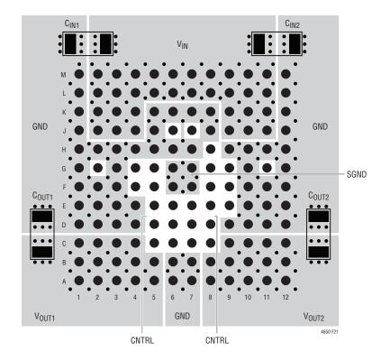
Figure 21. Recommended PCB Layout
