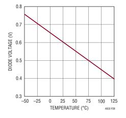
Figure 8. Diode Voltage  $V_D$  vs Temperature T(°C)
