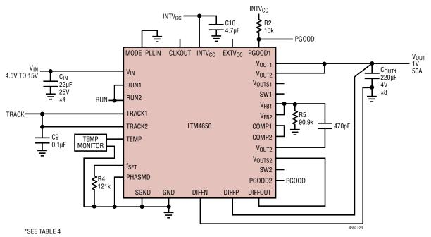
Figure 23. LTM4650 2-Phase, 1V at 50A Design
