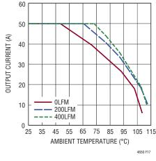
Figure 17. 5V to 1.5V Derating Curve, No Heat Sink
