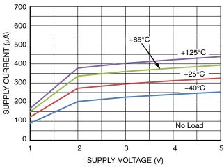
Figure 2. Quiescent Supply Current vs. Supply Voltage
