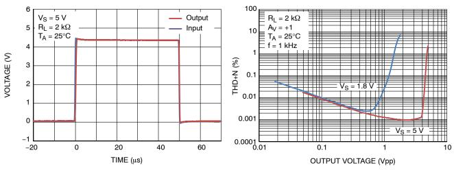
Figure 18. Non-Inverting Large Signal Transient Response
