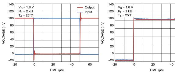
Figure 14. Inverting Small Signal Transient Response
