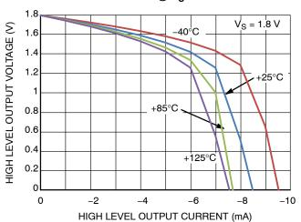
Figure 7. High Level Output Voltage vs. Output Current @  $V_S = 1.8 \text{ V}$
