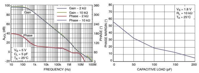
Figure 12. Open Loop Gain and Phase vs. Frequency @  $V_S = 5 \text{ V}$
