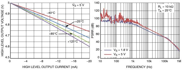
Figure 8. High Level Output Voltage vs. Output Current @  $V_S = 5 V$
