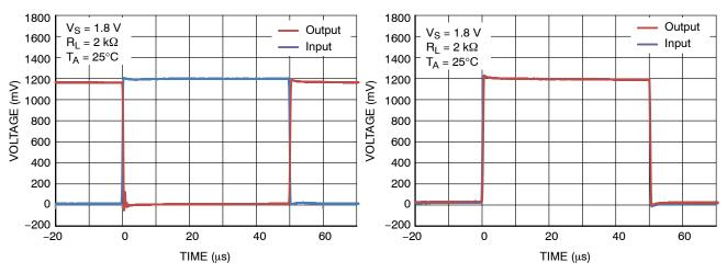
Figure 16. Inverting Large Signal Transient Response
