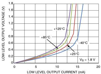
Figure 5. Low Level Output Voltage vs. Output Current @ V<sub>S</sub> = 1.8 V
