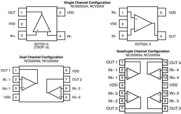
Figure 1. Pin Connections
