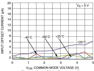
Figure 4. Input Offset Current vs. V<sub>CM</sub>
