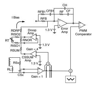
Figure 15. Droop Injection and Thermal Compensation
