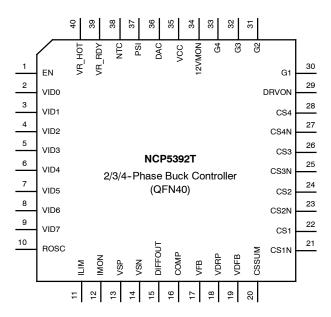
Figure 1. NCP5392T QFN40 Pin Connections (Top View)
