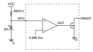
Figure 21. VRHOT Circuit
