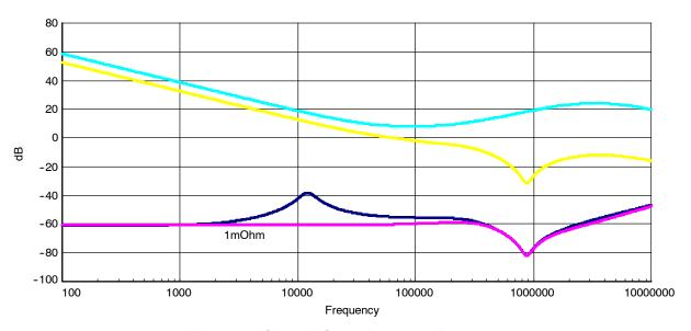
Figure 14. NCP5392T Circuit Frequency Response
