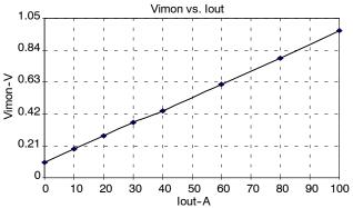
Figure 18. IMON Output vs. Output Current
