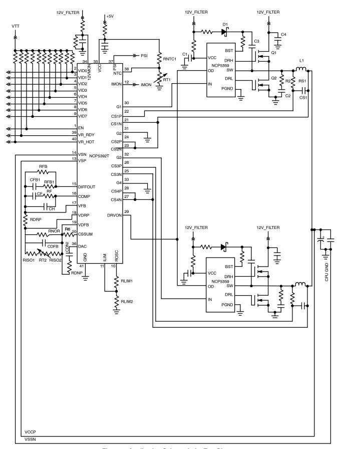
Figure 5. Application Schematic for Two Phases
