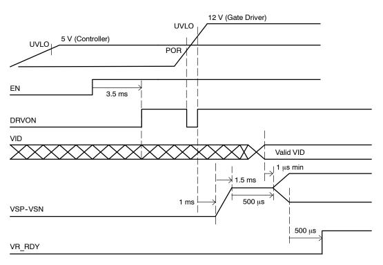
Figure 24. Driver UVLO Limited Startup
