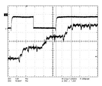
Figure 8. Dynamic VID Settling Time Rising (CH1: VID1, CH2: DAC, CH3:VCCP)
