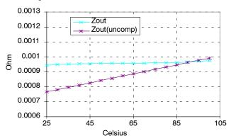
Figure 16. Zout vs. Temperature
