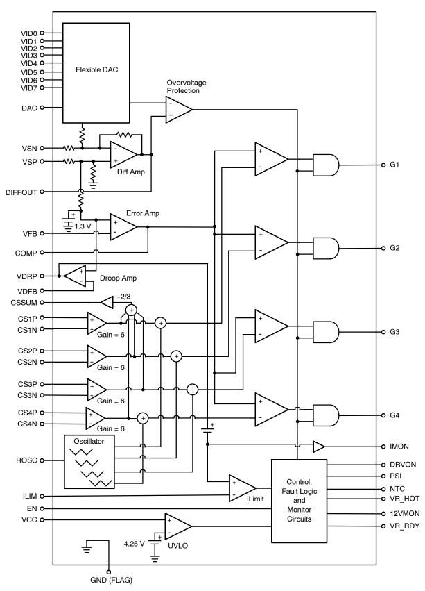
Figure 2. NCP5392T Block Diagram
