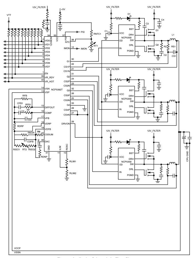
Figure 4. Application Schematic for Three Phases
