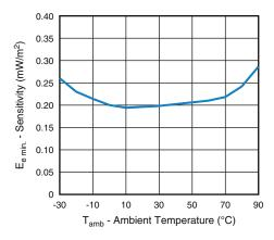
Fig. 9 - Sensitivity vs. Ambient Temperature
