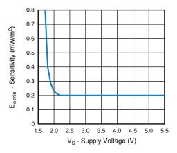
Fig. 12 - Sensitivity vs. Supply Voltage
