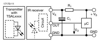
$R_1$  and  $C_1$  recommended to reduce supply ripple for  $V_S < 2.8 \text{ V}$
