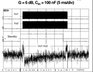
Figure 59. Startup and shutdown time  $V_{CC} = 5 V$ ,
