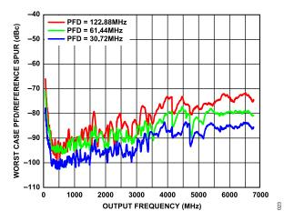
Figure 23. Worst Case PFD/Reference Spur vs. Output Frequency (RF<sub>OUT</sub>A+/ RF<sub>OUT</sub>A-), f<sub>PFD</sub> = 30.72 MHz, 61.44 MHz, and 122.88 MHz, Loop Filter = 3 kHz
