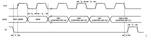
Figure 2. Write Timing Diagram
