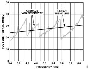
Figure 33. VCO Sensitivity, K<sub>V</sub> vs. Frequency
