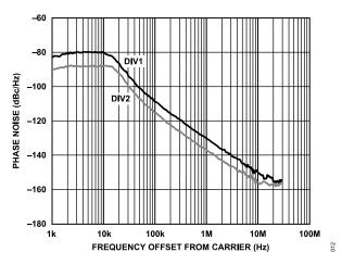
Figure 12. Closed-Loop Phase Noise, RF<sub>OUT</sub>A+, Fundamental VCO and Divide by 2, VCO = 6.8 GHz, f<sub>PFD</sub> = 61.44 MHz, Loop Bandwidth = 10 kHz
