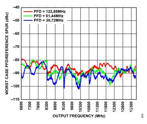
Figure 24. Worst Case PFD/Reference Spur vs. Output Frequency (RF<sub>OUT</sub>B), f<sub>PFD</sub> = 30.72 MHz, 61.44 MHz, and 122.88 MHz, Loop Filter = 3 kHz
