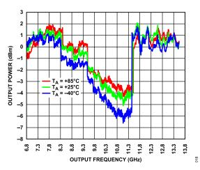
Figure 18. RF<sub>OUT</sub>B Output Power vs. Output Frequency (10 pF AC Coupling Capacitors, Board and Cable Losses De-Embedded)
