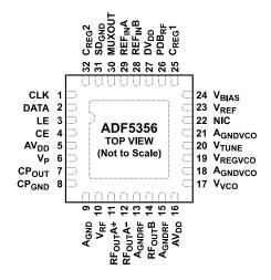
NOTES 1. NIC = NO INTERNAL CONNECTION. FOR EXISTING DESIGNS THAT CURRENTLY USE THE ADF5355, TO UPGRADE TO THE ADF5356, THE R<sub>SET</sub> RESISTOR CAN BE LEFT CONNECTED TO THIS PIN. 2. THE EXPOSED PAD MUST BE CONNECTED TO A<sub>GND</sub>.
