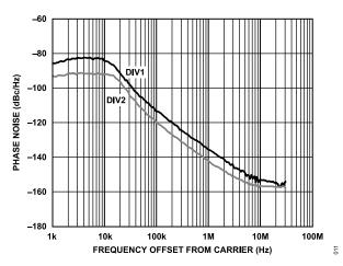
Figure 11. Closed-Loop Phase Noise, RF<sub>OUT</sub>A+, Fundamental VCO and Divide by 2, VCO = 5.0 GHz, f<sub>PFD</sub> = 61.44 MHz, Loop Bandwidth = 10 kHz
