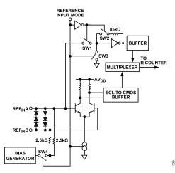
Figure 29. Reference Input Stage
