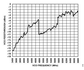
Figure 19. VCO Feedthrough at RF<sub>OUT</sub>B (Board and Cable Losses De-Embedded) vs. VCO Frequency
