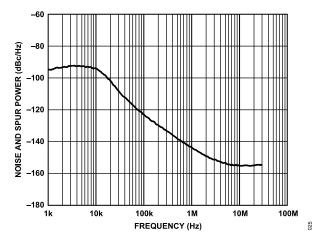
Figure 25. Fractional-N Spur Performance, GSM1800 Band, RF<sub>OUT</sub>A+ = 1550.2 MHz, f<sub>REFIN</sub> = 122.88 MHz, f<sub>PED</sub> = 61.44 MHz, Output Divide by 4 Selected, Loop Filter Bandwidth = 10 kHz, Channel Spacing = 20 kHz
