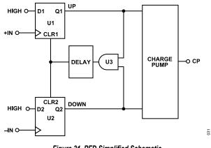
Figure 31. PFD Simplified Schematic
