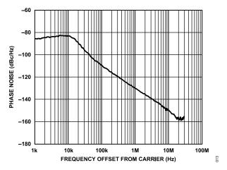
Figure 13. Closed-Loop Phase Noise, RF<sub>OUT</sub>B = 6.8 GHz, 2× VCO, VCO = 3.4 GHz, f<sub>PFD</sub> = 61.44 MHz, Loop Bandwidth = 10 kHz
