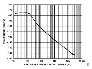
Figure 15. Closed-Loop Phase Noise, RF<sub>OUT</sub>B = 13.6 GHz, 2× VCO, VCO = 6.8 GHz, f<sub>PFD</sub> = 61.44 MHz, Loop Bandwidth = 10 kHz
