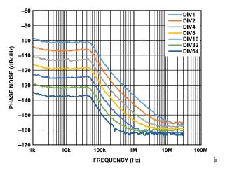
Figure 7. Closed-Loop Phase Noise, RF<sub>OUT</sub>A+ (100 nH Inductors), Fundamental VCO and Dividers, VCO = 3.4 GHz, PFD = 61.44 MHz, Loop Bandwidth = 40 kHz
