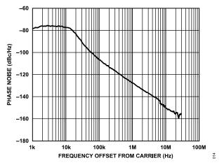
Figure 14. Closed-Loop Phase Noise, RF<sub>OUT</sub>B = 10 GHz, 2× VCO, VCO = 5.0 GHz, f<sub>PFD</sub> = 61.44 MHz, Loop Bandwidth = 10 kHz
