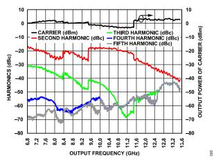
Figure 20. Harmonics and RF<sub>OUT</sub>B Output Power of Carrier vs. Output Frequency (10 pF AC Coupling Capacitors, Board and Cable Losses De-Embedded)
