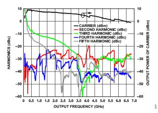
Figure 17. Harmonics and RF<sub>OUT</sub>A+/RF<sub>OUT</sub>A- Output Power of Carrier vs. Output Frequency (7.4 nH Inductors, 10 pF AC Coupling Capacitors, Board and Cable Losses De-Embedded)
