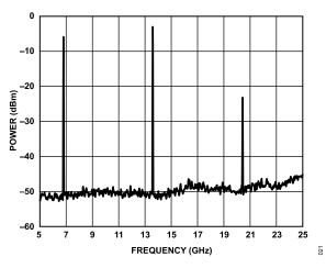
Figure 21. Wideband Spectrum, RF<sub>OUT</sub>B, VCO = 6.8 GHz, RF<sub>OUT</sub>B Enabled, RF<sub>OUT</sub>A+/RF<sub>OUT</sub>A- Disabled (Board Measurement)
