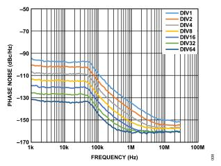
Figure 8. Closed-Loop Phase Noise, RF<sub>OUT</sub>A+ (100 nH Inductors), Fundamental VCO and Dividers, VCO = 5.0 GHz, PFD = 61.44 MHz, Loop Bandwidth = 40 kHz
