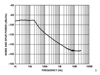
Figure 27. Fractional-N Spur Performance, RF<sub>OUT</sub>A+ = 2.591 GHz, f<sub>REFIN</sub> = 122.88 MHz, f<sub>PFD</sub> = 61.44 MHz, Output Divide by 2 Selected, Loop Filter Bandwidth = 10 kHz, Channel Spacing = 20 kHz
