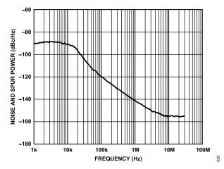
Figure 26. Fractional-N Spur Performance, W-CDMA Band, RF<sub>OUT</sub>A+ = 2113.5 MHz, f<sub>REFIN</sub> = 122.88 MHz, f<sub>PFD</sub> = 61.44 MHz, Output Divide by 2 Selected, Loop Filter Bandwidth = 10 kHz, Channel Spacing = 20 kHz
