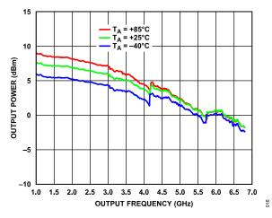
Figure 16. RF<sub>OUT</sub>A+/RF<sub>OUT</sub>A- Output Power vs. Output Frequency, (7.4 nH Inductors, 10 pF AC Coupling Capacitors, Board and Cable Losses De-Embedded)
