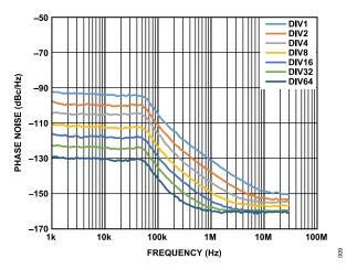
Figure 9. Closed-Loop Phase Noise, RF<sub>OUT</sub>A+ (100 nH Inductors), Fundamental VCO and Dividers, VCO = 6.8 GHz, PFD = 61.44 MHz, Loop Bandwidth = 40 kHz
