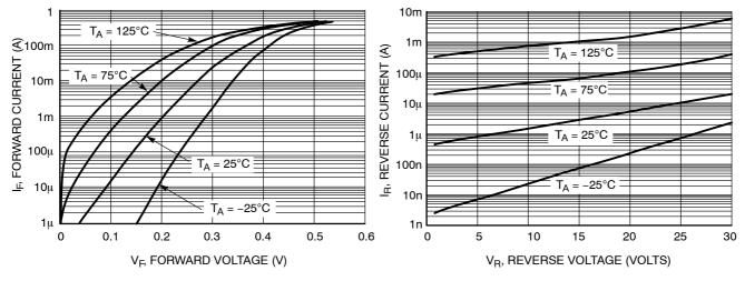
Figure 1. Forward Characteristics
