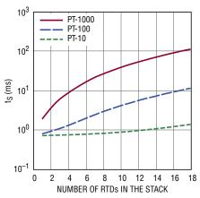
Figure 3. Simulated Settling Time of the RTD Stack
