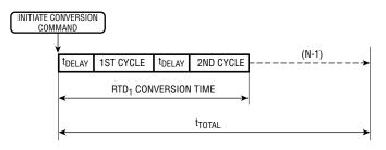
Figure 4. Total Conversion Time of the RTD Stack
