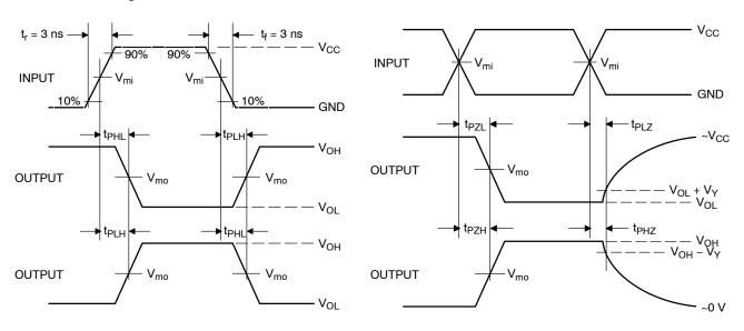
Figure 4. Switching Waveforms
