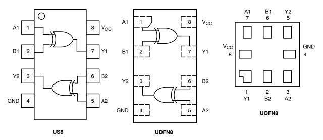
Figure 2. Pinout
