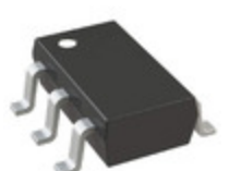
74V1G05STR STMicroelectronics IC INVERTER OD 1CH 1-INP SOT23-5
