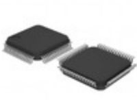
STM32F105R8T6 STMicroelectronics IC MCU 32BIT 64KB FLASH 64LQFP
