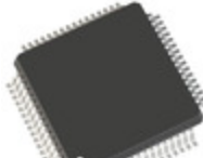
STM32F105R8T6TR STMicroelectronics IC MCU 32BIT 64KB FLASH 64LQFP
