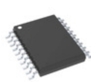
PIC16F631T-I/SS Microchip Technology IC MCU 8BIT 1.75KB FLASH 20SSOP
