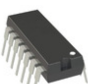
PIC16F630-I/P Microchip Technology IC MCU 8BIT 1.75KB FLASH 14DIP
