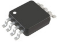
AD8131ARM Analog Devices Inc. IC OPAMP DIFF 1 CIRCUIT 8MSOP
