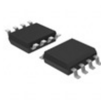
ATTINY45-15ST Microchip Technology IC MCU 8BIT 4KB FLASH 8SOIC
