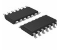
ATTINY44A-SSF Microchip Technology IC MCU 8BIT 4KB FLASH 14SOIC
