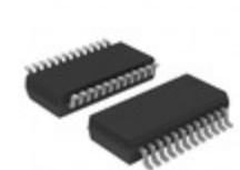
MCP3905AT-I/SS Microchip Technology IC POWER METERING-1 PHASE 24SSOP
