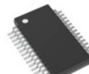
MCP3919A1-E/SS Microchip Technology IC ENERGY METER FRONT 3CH 28SSOP
