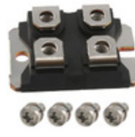
STTH200R04TV1 STMicroelectronics DIODE MODULE 400V 100A ISOTOP
