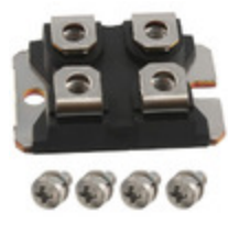
STTH200F04TV1 STMicroelectronics DIODE GEN PURP 400V 100A ISOTOP
