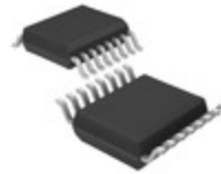
ADM1031ARQZ-R7 onsemi IC SENSOR 2TEMP/FAN CTRL 16QSOP
