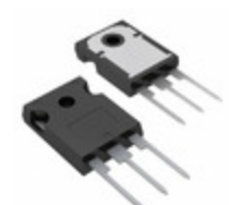
STW40N90K5 STMicroelectronics MOSFET N-CH 900V 40A TO247
