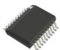
AD73311LARS Analog Devices Inc. IC ANALOG FRONT END 20-SSOP
