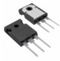
STGW30V60DF STMicroelectronics IGBT 600V 60A 258W TO247
