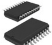
ST7FLITE39F2M3 STMicroelectronics IC MCU 8BIT 8KB FLASH 20SO
