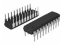
ST7FLITE25F2B6 STMicroelectronics IC MCU 8BIT 8KB FLASH 20DIP
