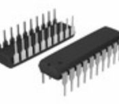
ST7FLITE35F2B6 STMicroelectronics IC MCU 8BIT 8KB FLASH 20DIP
