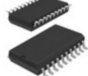
ST7FLITE15M6TR STMicroelectronics IC MCU 8BIT 4KB FLASH 20SOIC
