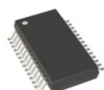
AD977ACRSZ Analog Devices Inc. IC ADC 16BIT SAR 28SSOP
