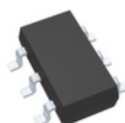
24AA025E48T-E/OT Microchip Technology IC EEPROM 2KBIT I2C SOT23-6
