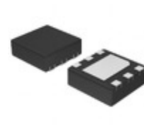
CAT6219ADJVP5GT4 onsemi IC REG LIN POS ADJ 500MA 6TDFN
